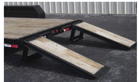
Wood Filled Ramps
